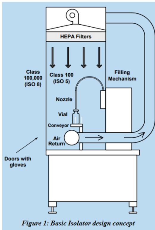
and sterilized in place. In addition to accommodating lyophilized vials, isolator technology offers Lyophilization capability. Isolator provided high level of assurance to maintain your product sterility. Gloves leakages play a major role for breaching integrity of isolator and potential cause for sterility failure.
